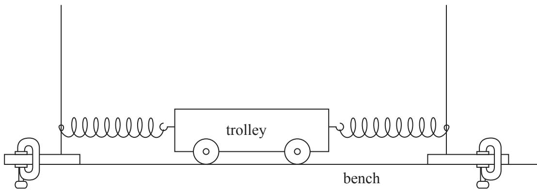
When pulled to one side and released, the trolley oscillates with simple harmonic motion. The periodic time  $T$  of this oscillation is measured. Masses  $m$  are placed on the trolley and the new periodic times are measured. The results are shown in the table.
